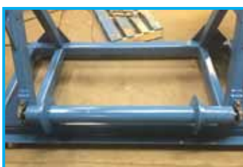
*OPTIONAL GUIDE ROLLER SHOWN REVERSING, 5.5 RPM / 6,000 LB. CAPACITY VOLTAGE: 240 / 480
