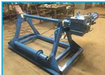
FIXED FRAME / 48" BELT WIDTH 3 PHASE MOTOR / 3 HP ELECTRIC DRIVE w / BRAKE
