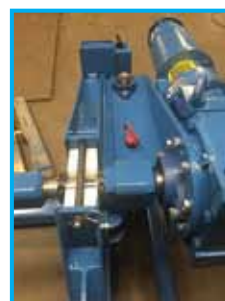
3" SQUARE CORE BAR UHMW PILLOW BLOCKS / SAFETY PINS SELF-CONTAINED HYDRAULIC DRIVE
