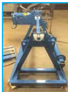
3" SQUARE CORE BAR UHMW PILLOW BLOCKS / SAFETY PINS SELF-CONTAINED HYDRAULIC DRIVE
