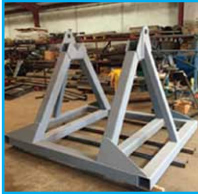
REINFORCED GUSSETED SUPPORTS
