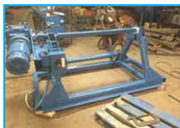
FIXED FRAME / 48" BELT WIDTH 3 PHASE MOTOR / 3 HP ELECTRIC DRIVE w / BRAKE
